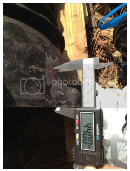
$\circ$   $\;$   $\;$  From the center of the volt hole, measure up 36mm to intersect the first line
