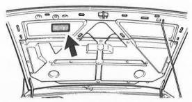
The Vehicle Emission Control Information (VECI) label is located on the under side of the hood
