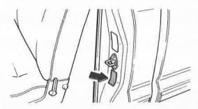
The tire pressure label can be found on the driver's side door pillar
