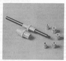
Clutch plate alignment tool
