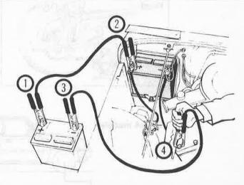
Make the booster battery cable connections in the numerical order shown (note that the negative cable of the booster battery is NOT attached to the negative terminal of the dead battery)
