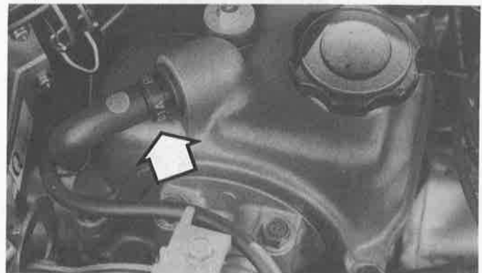
43.2 The PCV valve (arrow) is located in the rocker cover on these models (1988 and later model shown).
