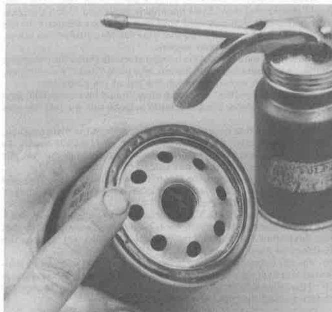
12.18 Lubricate the oil filter gasket with clean engine oil before installing the filter on the engine
