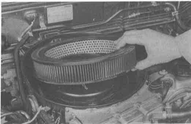
29.4 After the top plate has been removed from the air cleaner housing, lift the air filter out of position — be careful not to drop any dirt, tools, etc. down the center of the carburetor
