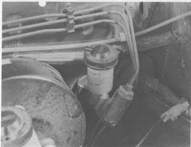
4.19b The clutch fluid level should be kept between the Max and Min marks on the reservoir
