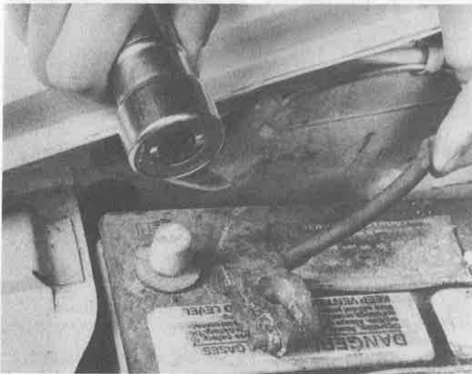
8.7c Regardless of the type of tool used to clean the battery posts, a clean, shiny surface should be the result
