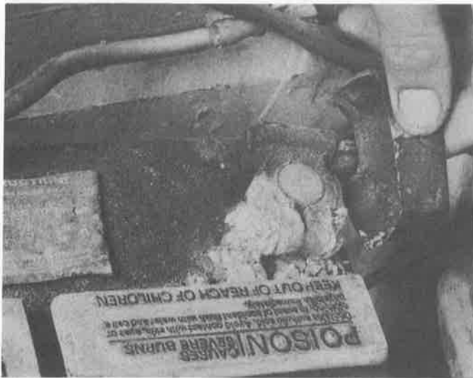
8.7a Battery terminal corrosion usually appears as light fluffy powder
