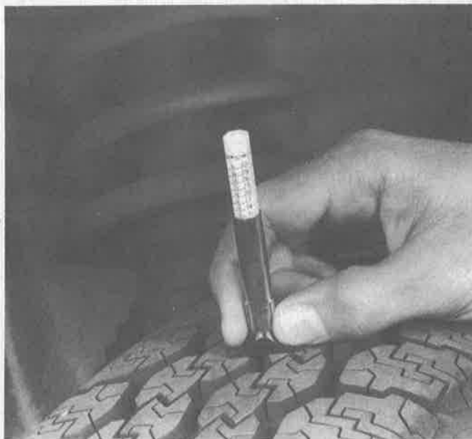
7.2 A tire wear tread depth indicator should be used to monitor tire wear — they are available at auto parts stores and service stations and cost very little
