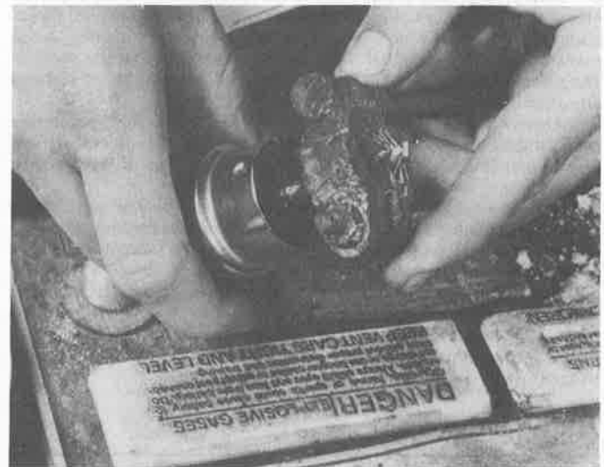
8.7d When cleaning the cable clamps, all corrosion must be removed (the inside of the clamp is tapered to match the taper on the post, so don't remove too much material)
