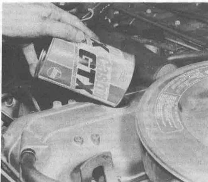
4.6 After unscrewing the filler cap from the rocker arm cover, oil can be added to the engine
