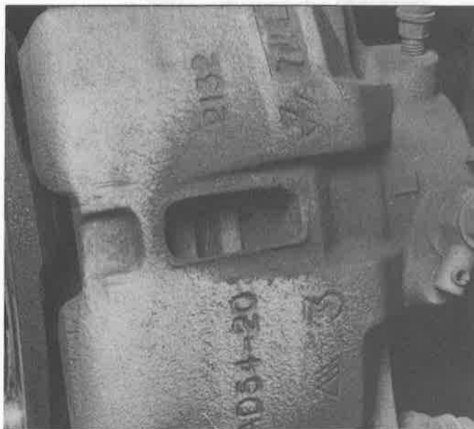
24.5 The disc brake pads are visible through the opening slot in the caliper
