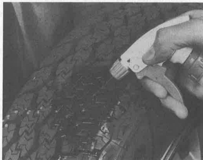
7.4b If the valve core is tight, raise the corner of the vehicle with the low tire and spray a soapy water solution onto the tread as the tire is turned slowly — slow leaks will cause small bubbles to appear
