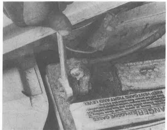
8.7b Removing a cable from the battery post with a wrench — sometimes a special battery pliers is required for this procedure if corrosion has caused deterioration of the nut hex (always remove the ground cable first and hook it up last!)
