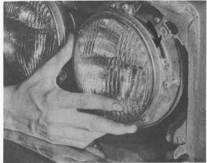
10.2b . . . rotate the bezel to line up the screw "keyhole" slots and pull it off
