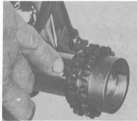
10.7 Install the timing chain sprocket on the end of the crankshaft with the wide shoulder facing out
