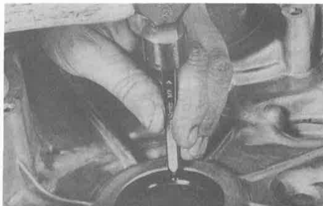
13.8 Drive the old oil seal out of the timing chain cover with a hammer and punch
