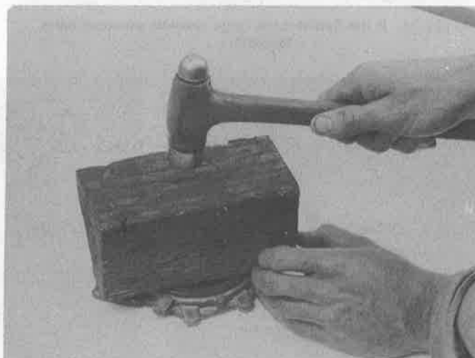
22.15 Drive the new seal into the housing with a block of wood — make sure you don't cock the seal
