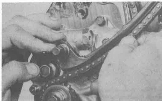
13.6 Adjusting the balance shaft chain slack (1988 and earlier 2.6L engine)
