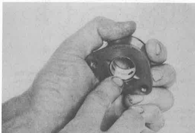
14.7 Checking the bearing in the thrust plate for wear and damage
