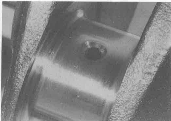
18.4 Check the oil holes in the crankshaft journals to make sure they're clean and smooth — sharp edges here will damage the new bearings!
