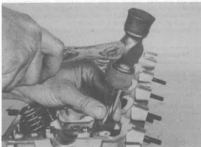
11.4a Install the new valve guide seals with a hammer and deep socket — don't hammer on the seals once they're seated!
