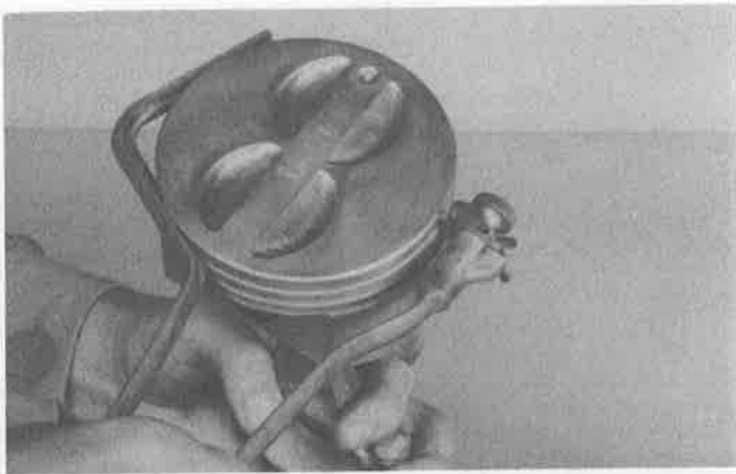
17.4a The piston ring grooves can be cleaned with a special tool, as shown here, . . .
