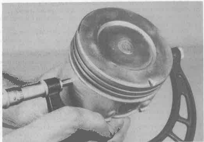
17.11 Measure the piston diameter at the specified point, at right angles to the piston pin
