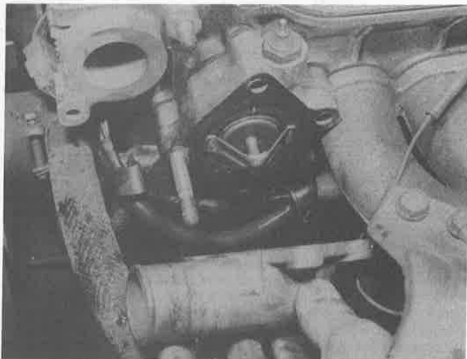
3.9b On pre-1985 models, the thermostat housing is located at the front of the engine on the intake manifold side
