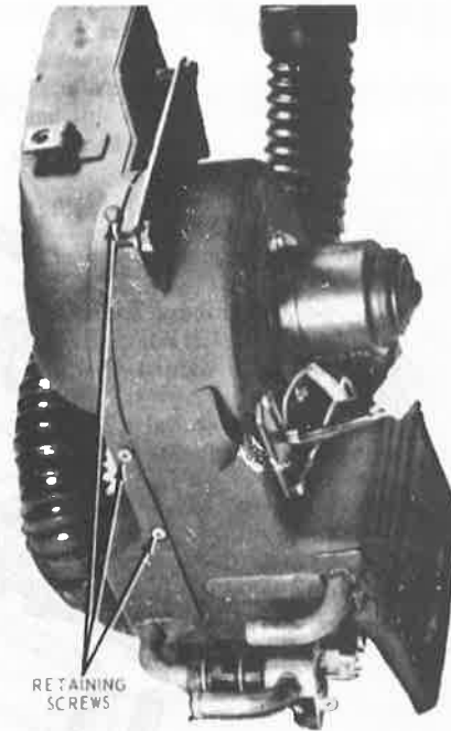
11.7 Remove the retaining screws to separate the case for access to the heater core (early model shown)
