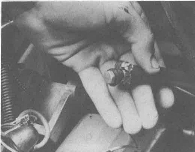
7.3 To plug rubber fuel hoses effectively, insert a bolt into the opening and secure it with a small hose clamp
