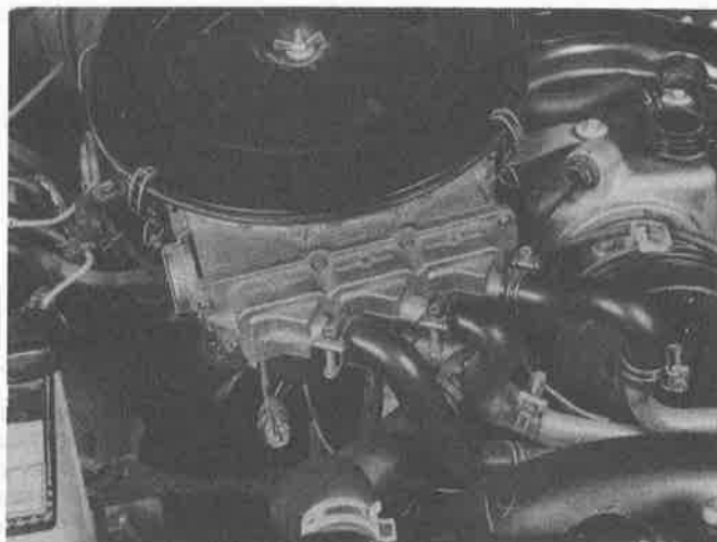
8.3 Late model vehicles have numerous hoses which must be detached from the air cleaner housing, including the three large hoses shown here. Using tape, label all hoses before disconnecting them. Also visible in this photo are the top cover securing clips and center wing nut.
