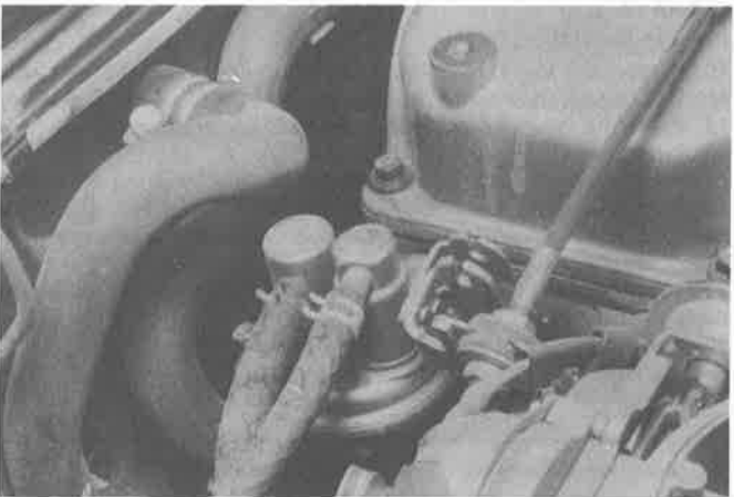
7.2 On some vehicles, a mechanical fuel pump is located on the cylinder head – when replacing the fuel pump, always use new gaskets
