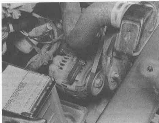
11.4 This view shows the alternator adjustment bolt, which is within the slotted portion of the bracket. The pivot bolt runs through a flange at the bottom of the alternator
