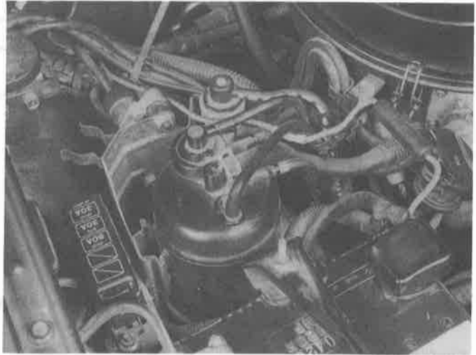
4.2b The charcoal cannister is located next to the battery and can be identified by the many vacuum hoses attached to it
