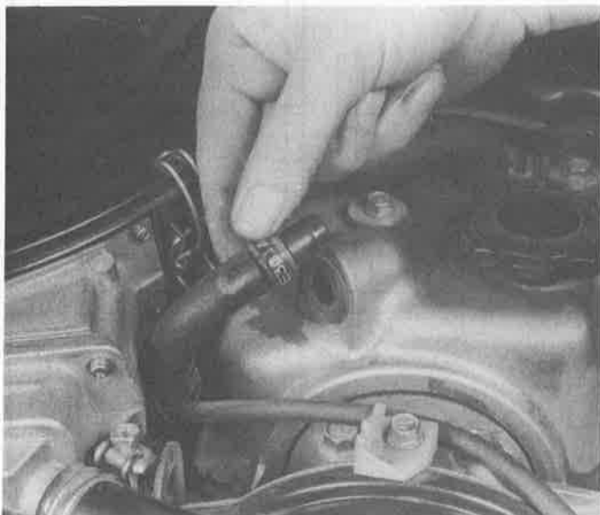
2.8a Removing the PCV valve and hose from the cylinder head
