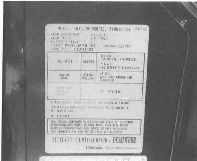
1.5a A typical Vehicle Emissions Control Information (VECI) label
