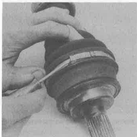
22.3b The boot clamps can be pried open with a small screwdriver
