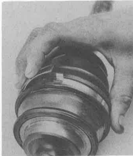
22.21a To install a new clamp, bend the tang downward and ...
