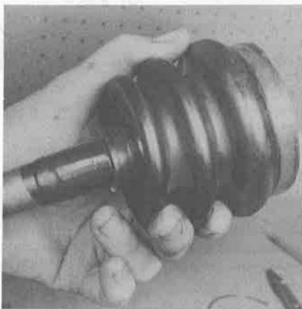
22.14 Wrap the splined area of the axle with tape to prevent damage to the boot when installing it
