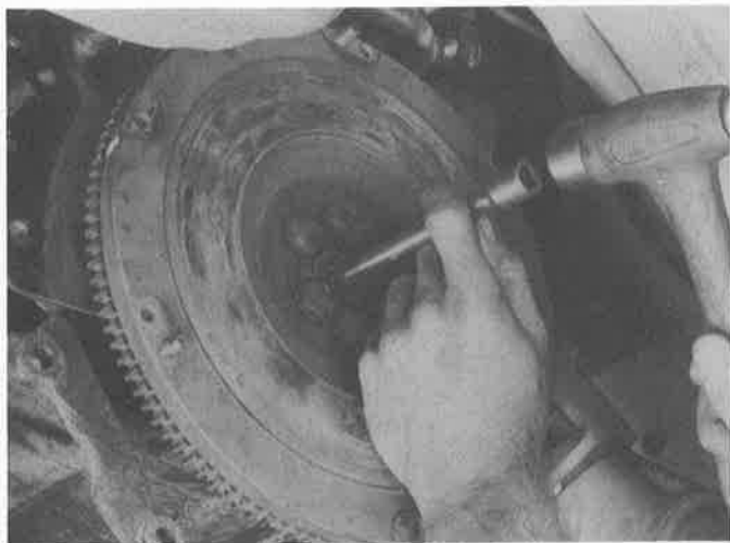
5.10 ... then force the bearing out hydraulically with a steel rod slightly smaller than the bore in the bearing — when the hammer strikes the rod, the grease will transmit force to the backside of the bearing and push it out
