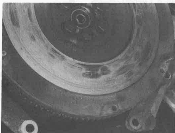
3.8 Check the flywheel for cracks, hot spots and other obvious defects (slight imperfections can be removed by a machine shop)
