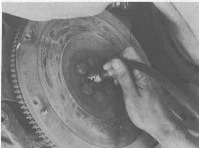
5.9 Fill the cavity behind the pilot bearing with grease . . .
