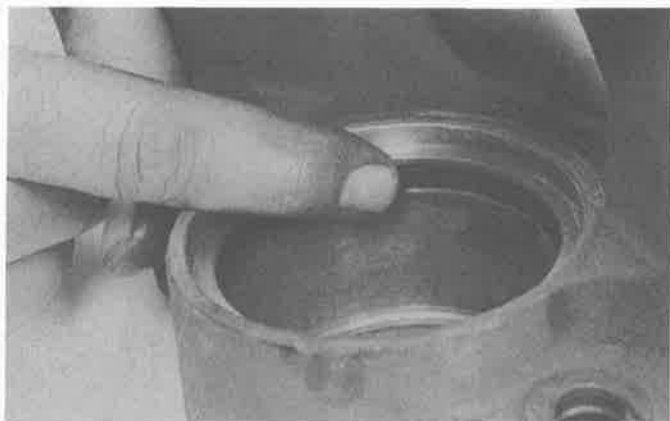
3.14 Position the seal in the caliper bore groove, making sure it isn't twisted
