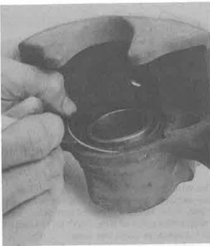
3.7a Using a screwdriver, remove the boot set ring
