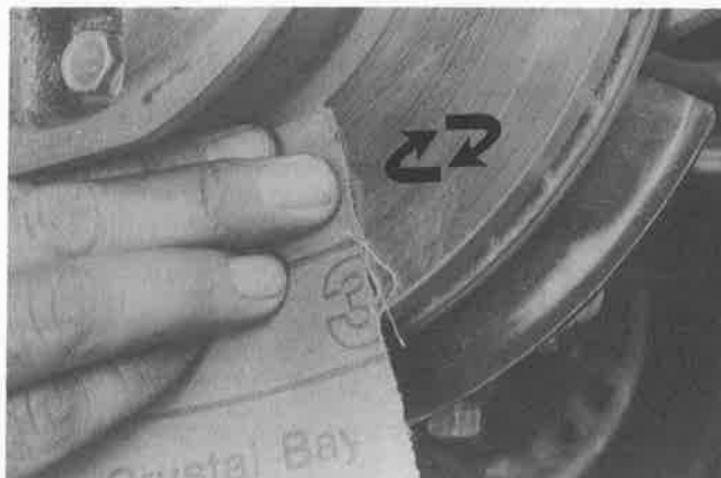
4.4b Using a swirling motion, remove the glaze from the disc with sandpaper or emery cloth
