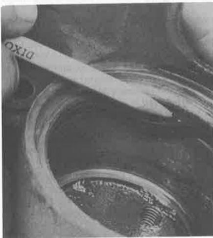
3.9 Because metal tools may cause damage, a wooden or plastic tool should be used to dig the piston seal out of its groove (a sharp pencil works well)
